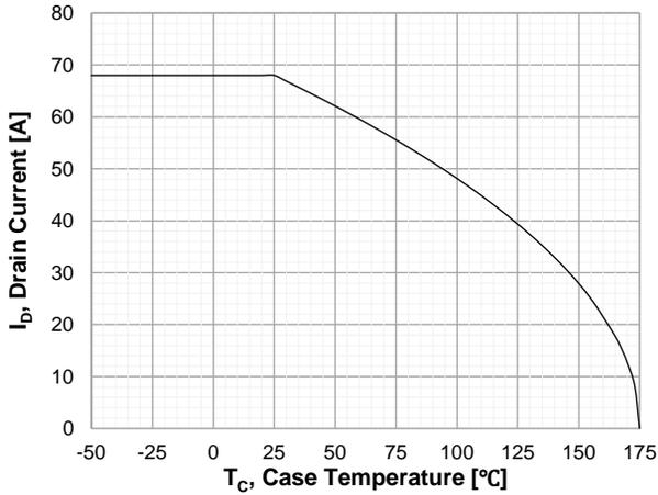
Figure 14. Maximum Power Dissipation Derating vs. Case Temperature
