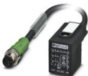
Sensor/actuator cable, 3-position, PUR halogen-free, yellow, Plug straight M12, A-coded, on Valve connector BI (11 mm), with 1 LED, connected with Z diode, cable length: 3 m
