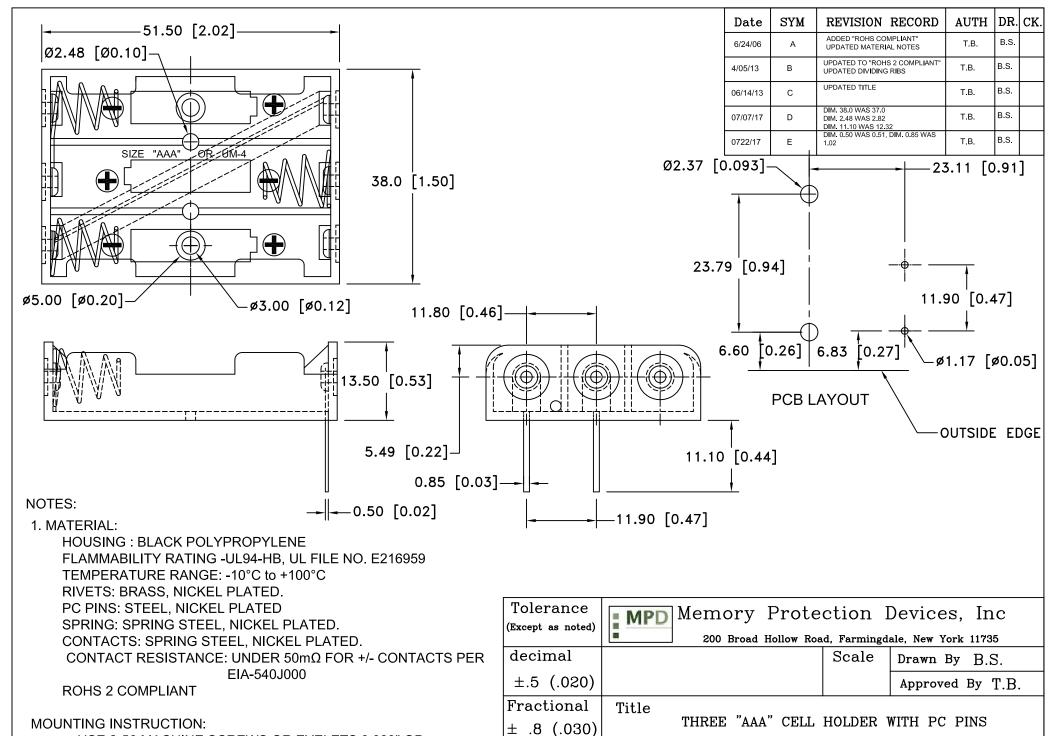
USE 2-56 MACHINE SCREWS OR EYELETS 0.089" OD BY 0.15" FLANGE STIMPSON GS-3 SERIES OR EQUIVALENT. ALSO ADHESIVES AND DOUBLE SIDED TAPES WORK WELL.
