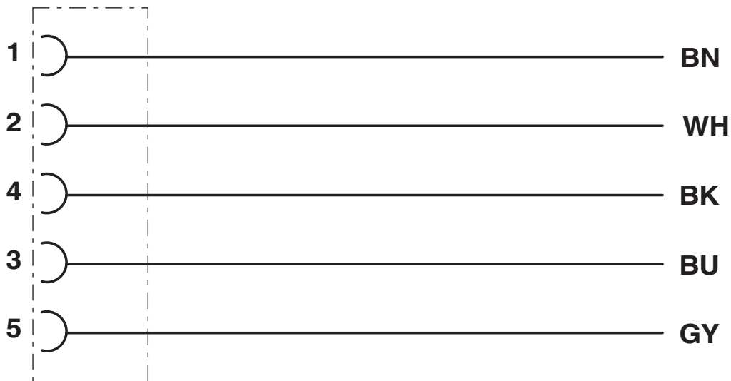
Contact assignment of the M12 socket
