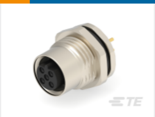
TE Part #T4141412041-000 M12,REAR MOUNTING,FEMALE,B CODE,4P
