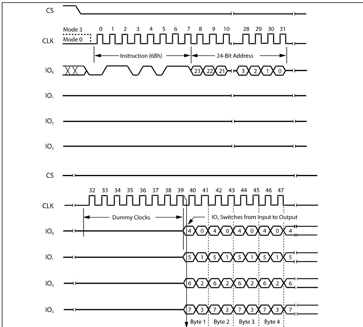
Figure 11. Fast Read Quad Output Instruction Sequence Diagram
