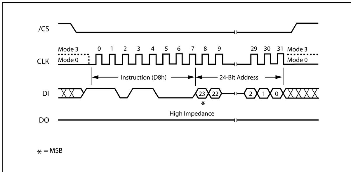
Figure 19. 64KB Block Erase Instruction Sequence Diagram
