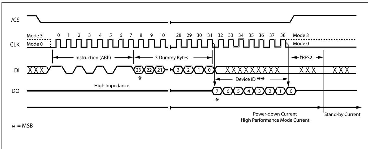
Figure 26. Release Power-down / Device ID Instruction Sequence Diagram
