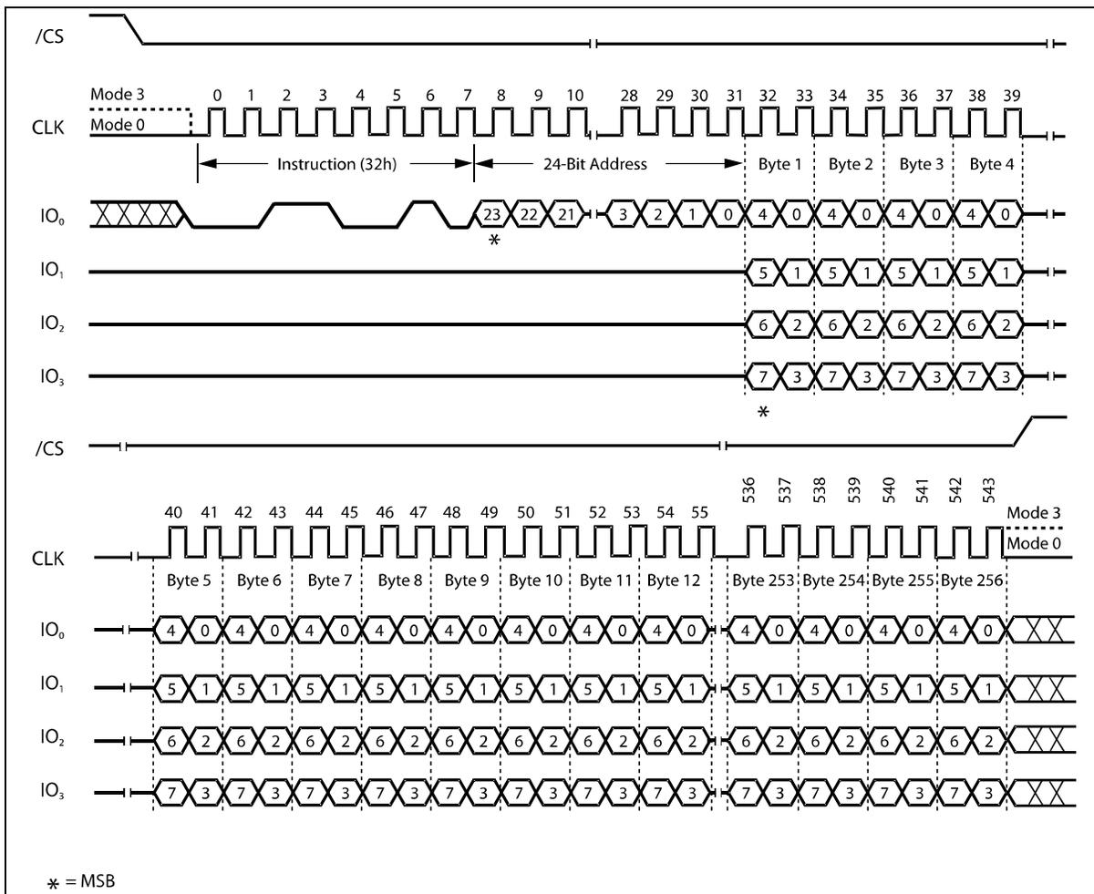
Figure 16. Quad Input Page Program Instruction Sequence Diagram
