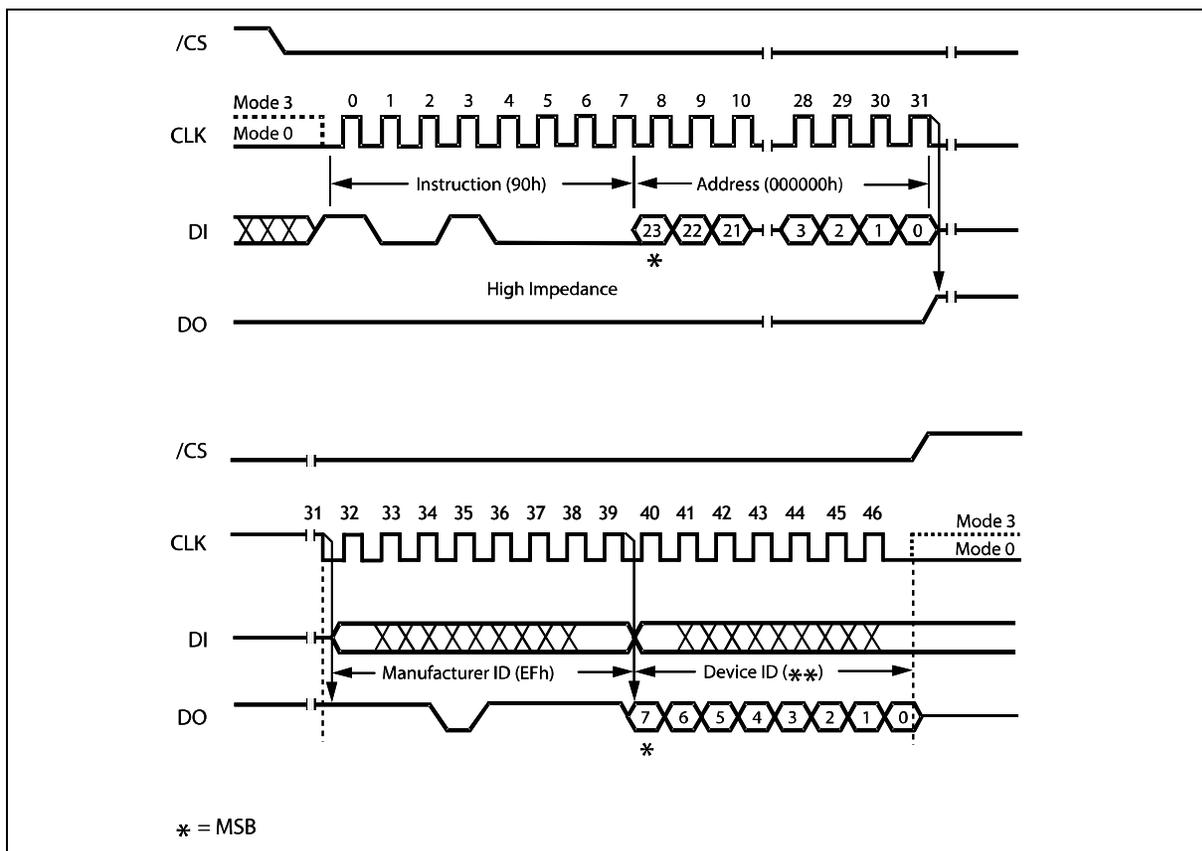
Figure 27. Read Manufacturer / Device ID Diagram
