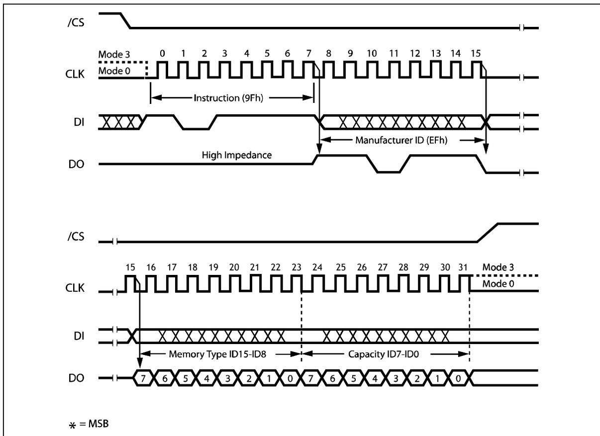
Figure 29. Read JEDEC ID Instruction Sequence Diagram
