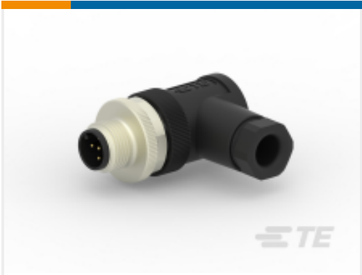
TE Part #T4113001051-000 M12,MALE,RA,A CODE,5P,PG7,GOLD
