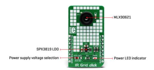
The MLX90621ESF-BAD IR sensor used on this Click board™ offers 40° x 10° FOV, with the IR sensing elements arranged in a 4x16 grid. Each sensor measures the temperature in its individual FOV, allowing the host MCU to build a thermal image or calculate the temperature at each spot of the imaged scene. The measurement results are stored in the onboard RAM. 64 words, each 16 bits wide contains the result of the IR sensor measurements, and one word contains the PTAT measurement.
