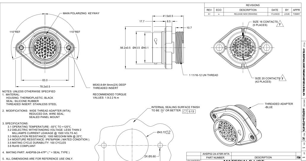
CONTACT MIN. INSUL MAX. INSUL TYPICAL WIRE CURRENT SIZE O.D. O.D. RANGE RATING 1.02 mm 2.10 mm 16-22 AWG 7.5 AMPS 20 (.040 in) (.083 in) (1.5-0.35mm<sup>2</sup>) 1.35 mm 2.62 mm 14-20 AWG 13 AMPS 16 (.053 in) (.103 in) (2.0-0.5mm<sup>2</sup>)
