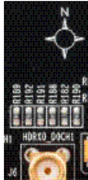
Figure C.1. CFG[2:0] Setting Resistor Field – Revision A
