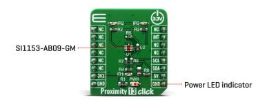
By default, the measurement parameters are optimized for indoor ambient light levels, where it is possible to detect low light levels. For operation under direct sunlight, the ADC can be programmed to operate in a high signal operation so that it is possible to measure direct sunlight without overflowing.
