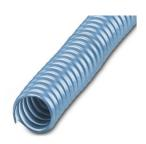
Protective hose, material: PU, filament: PUR sheathed spring steel, UV-resistant: no, flexible, degree of protection: IP68, color: blue, flammability rating in acc. with UL 94: V2, inner diameter: 38 mm, Total length: 10 m
