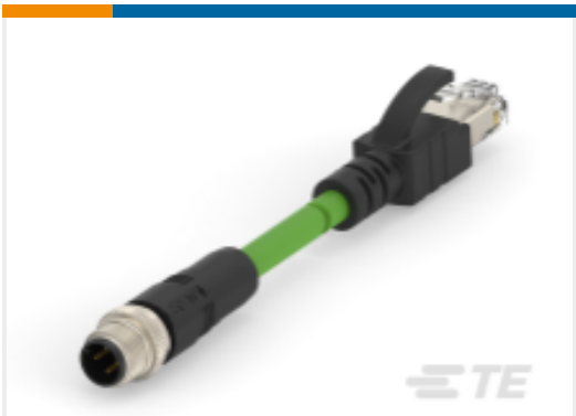
TE Part #TCD14745101-003 M12 D-code 4pin Male to RJ45 Cable Assembly, Cat5e Polyurethane 24AWG Shielded
