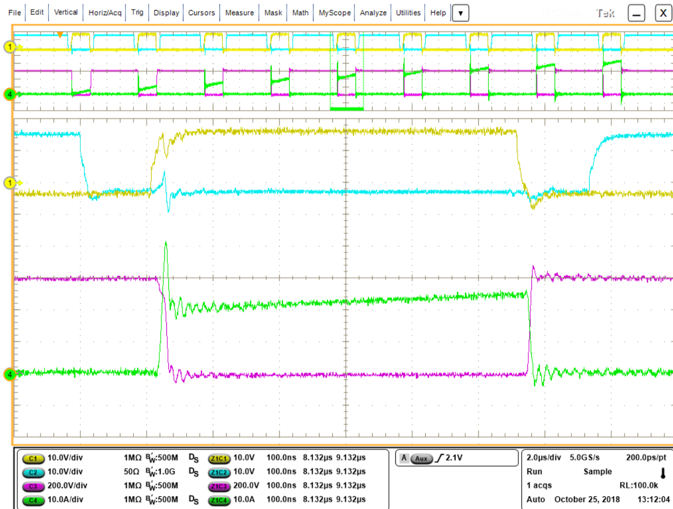
Figure 43. SiC MOSFET Switching Waveforms
