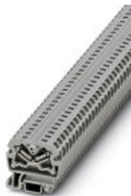
Mini feed-through terminal block, Connection method: Spring-cage connection, Cross section: 0.08 mm 2 - 4 mm 2 , AWG: 28 - 12, Width: 5.2 mm, Height: 22 mm, Color: blue, Mounting type: NS 15
