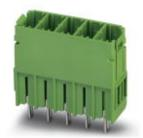
Header, Nominal current: 41 A, Rated voltage (III/2): 630 V, Number of positions: 10, Pitch: 7.62 mm, Color: green, Contact surface: Tin, Mounting: Soldering
