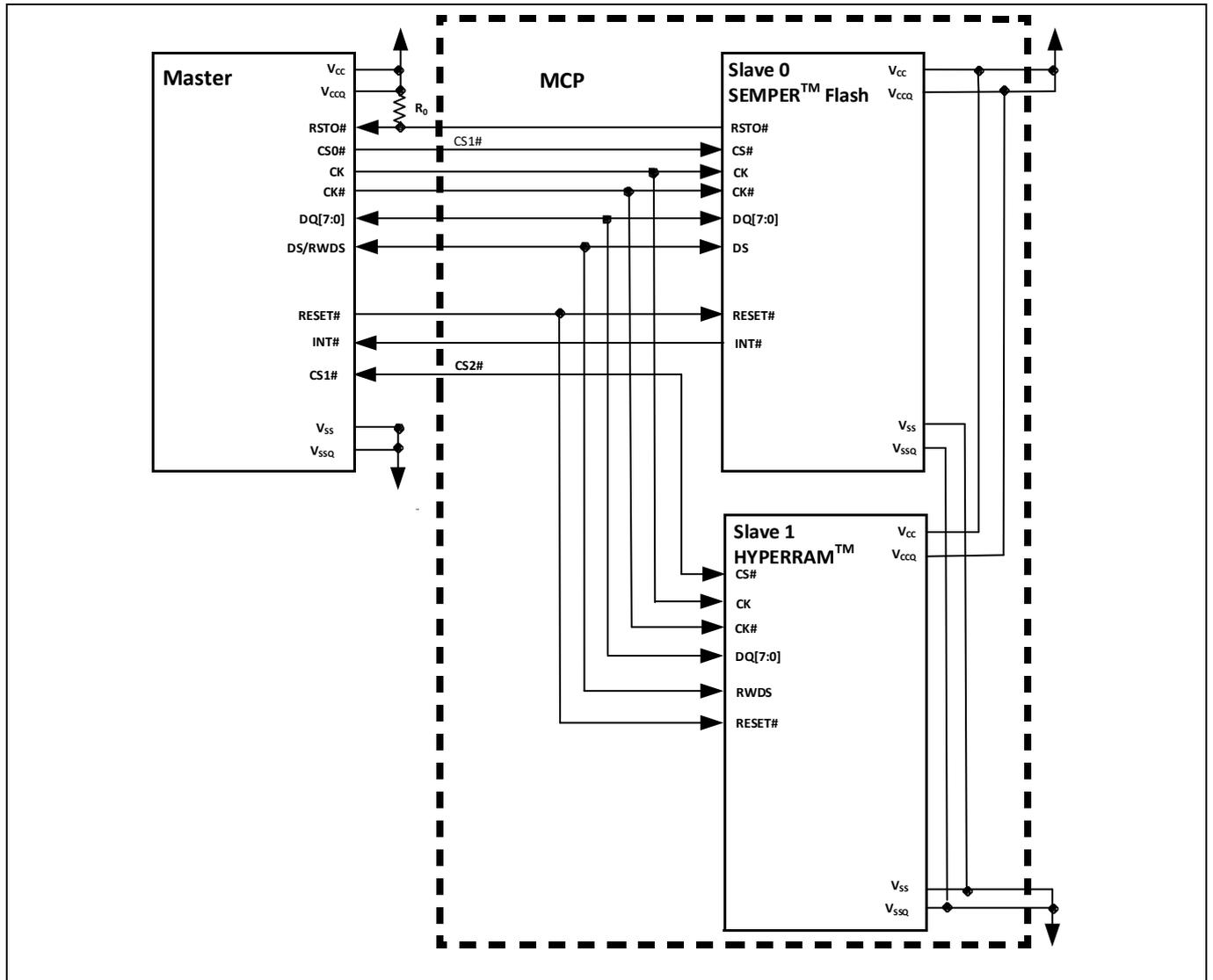
Figure 2 HYPERBUS™ connections including optional signals
