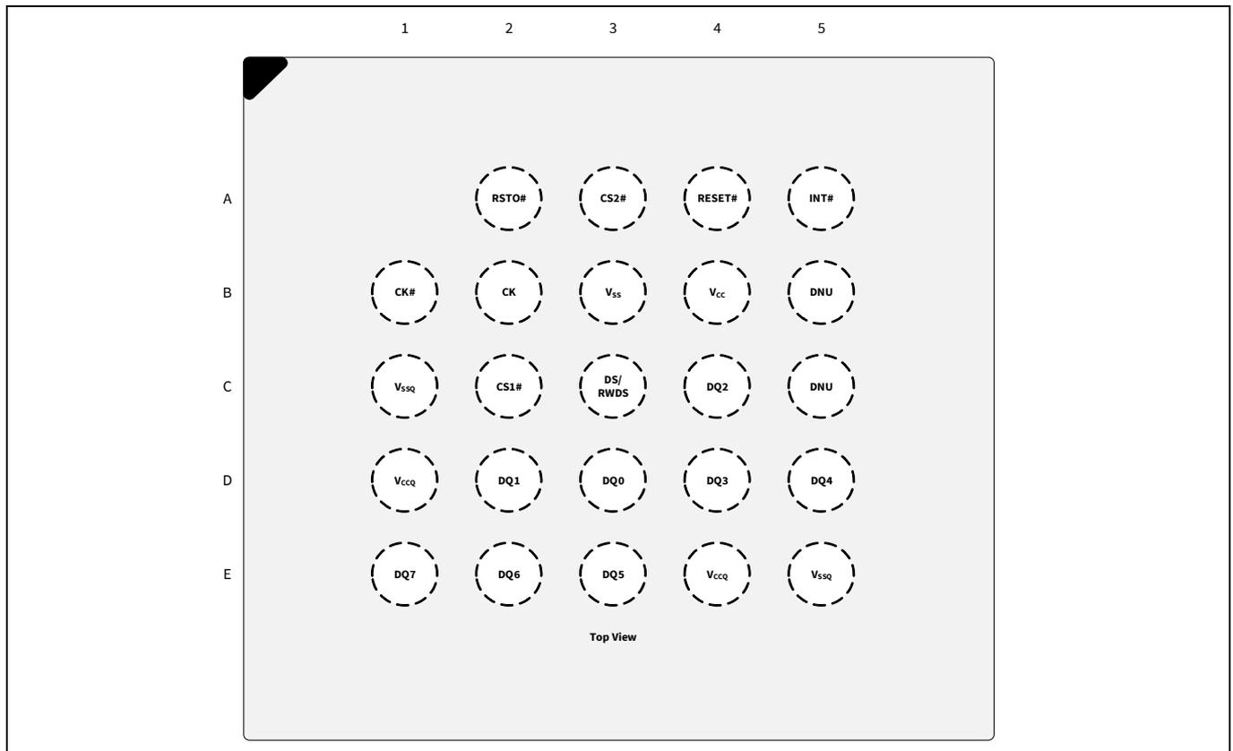
**Figure 3** 24-ball FBGA, 8 × 8 mm, 5 × 5 ball footprint (top view)
