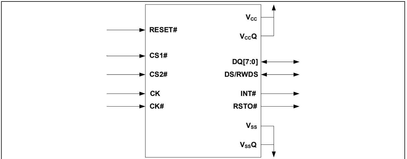
Figure 1 HYPERBUS™ MCP signal diagram
