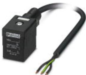
Sensor/Actuator cable, 3-position, PUR, black, free cable end, on Valve connector BI (11 mm), with 1 LED, connected with Damping diode, Cable length: 3 m, With holding current limiting device for energy reduction
