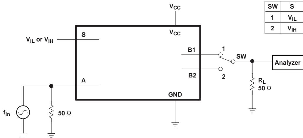
**Figure 8. Feedthrough**
