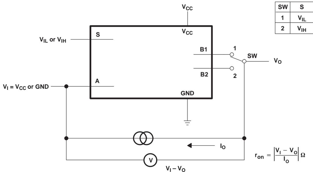
Figure 2. ON-State Resistance Test Circuit
