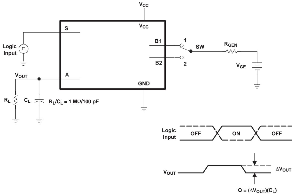
**Figure 9. Charge-Injection Test**
