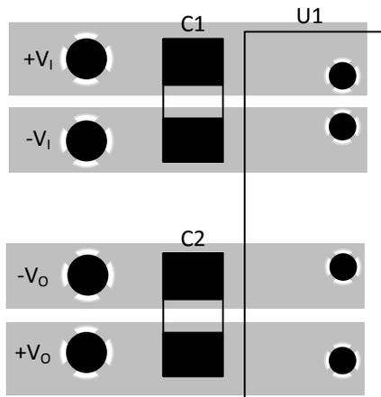
Figure 30. DCH01 Single Output Layout (Component-Side View)
