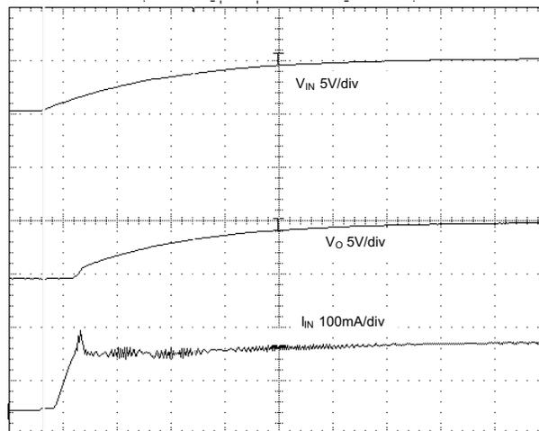
Figure 24. Startup Waveforms
