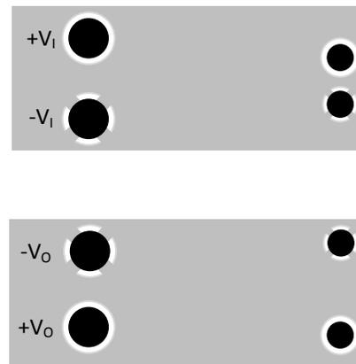
Figure 31. DCH01 Single Output Layout (Non-Component-Side View)
