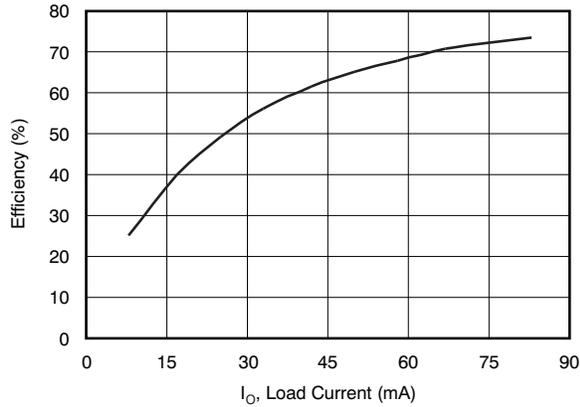
Figure 7. DCH010512S Efficiency
