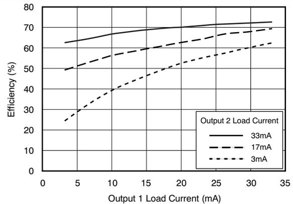
Figure 14. DCH010515D Efficiency
