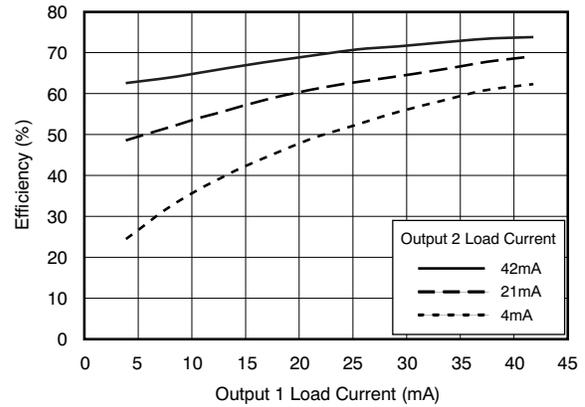
Figure 8. DCH010512D Efficiency
