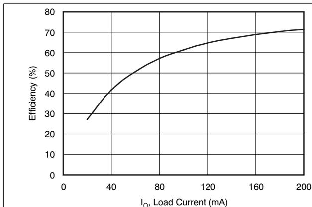
Figure 28. DCH010505S Efficiency
