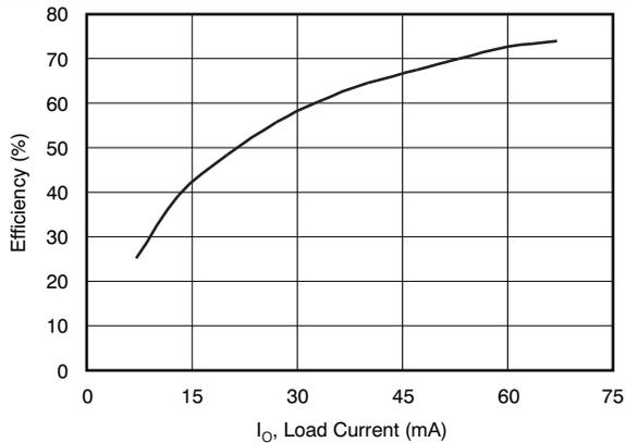
Figure 13. DCH010515S Efficiency
