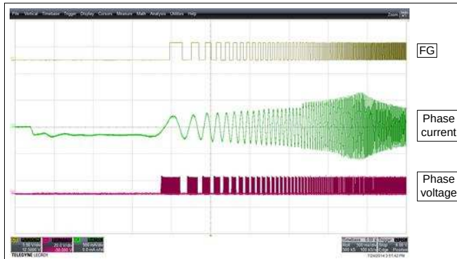
Figure 71. DRV10987 Start-Up Waveform
