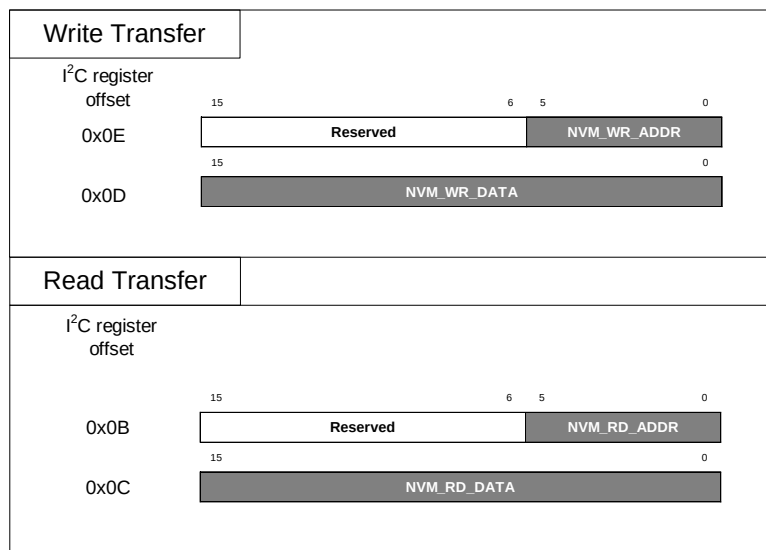
Figure 31. EEPROM Direct Access Using I 2 C
