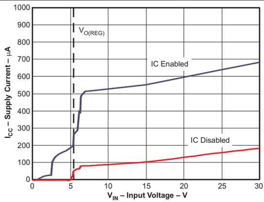
**Figure 8. Supply Current vs Input Voltage (bq24380)**
