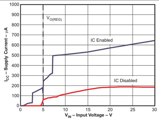
**Figure 9. Supply Current vs Input Voltage (bq24381)**
