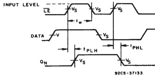
Fig. 4 - Latch enable propagation delays.
