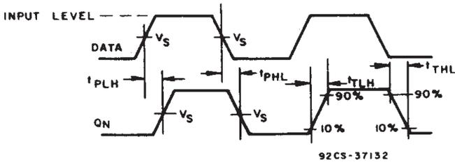
Fig. 3 - Data to  $Q_n$  output propagation delays and output transition times.
