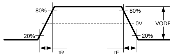
Figure 1. Driver Output Transition Time
