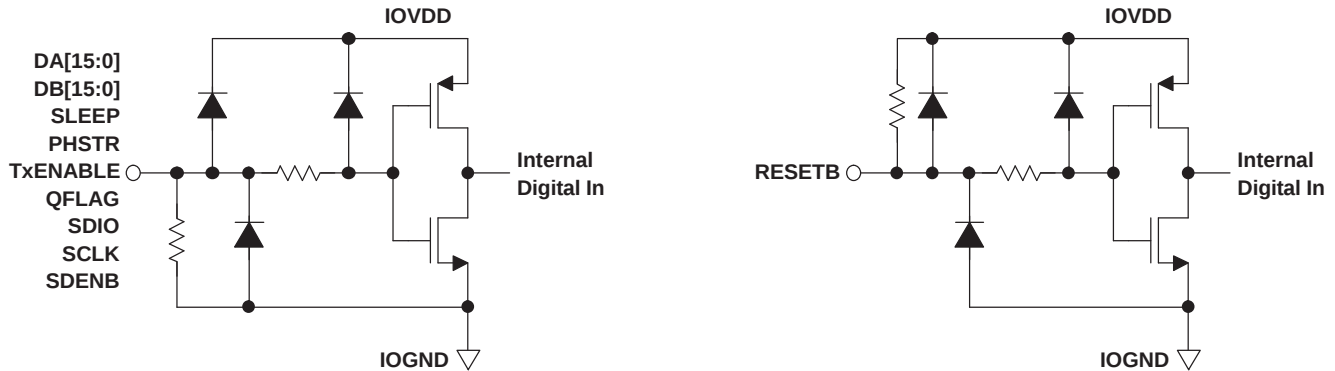
Figure 61. CMOS/TTL Digital Equivalent Input
