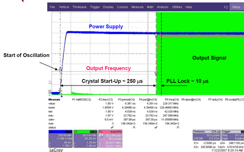
Figure 16. Crystal Oscillator Start-Up vs PLL Lock Time
