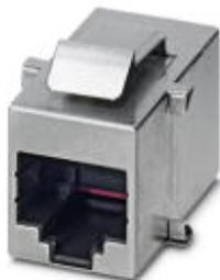
RJ45 coupling, Degree of protection: IP20, Number of positions: 8, 1 Gbps, CAT5 (IEC 11801:2002), Material: Fiberglass, PBT, Connection method: Female, Keystone
