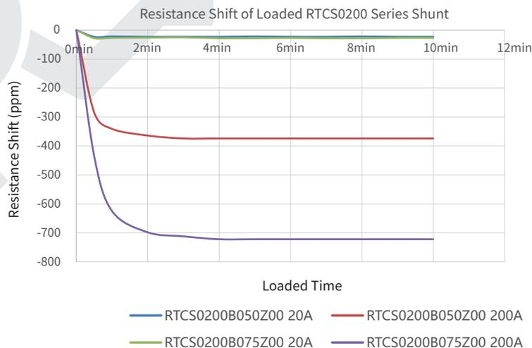
\*Under different heat dissipation conditions and different applied copper bar sizes, there will be some differences in the change of shunt on resistance. The above operating conditions are under normal temperature with 100mm<sup>2</sup> copper wire; For customized test, please contact us to provide detailed operating conditions.
