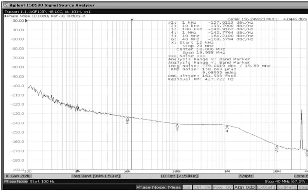
Figure 1. LVPECL Output (156.25MHz), 12kHz–20MHz Integration Bandwidth, 162fs Jitter, All Outputs Active
