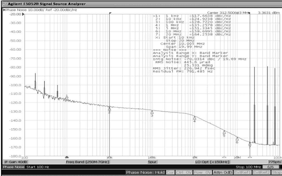
Figure 3. LVPECL Output (312.5MHz), 12kHz–20MHz Integration Bandwidth, 227fs Jitter, All Outputs Active
