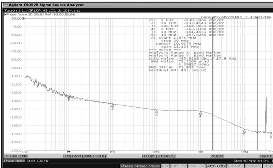
Figure 2. LVPECL Output (156.25MHz), 1.875MHz–20MHz Integration Bandwidth, 73fs Jitter, All Outputs Active
