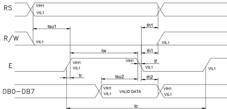
Read cycle ( $T_a=25^\circ\text{C}$ ,  $V_{DD}=5.0\text{V}$ )
