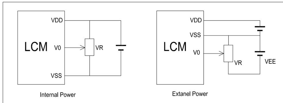
$V_{DD}-V_0$ : LCD Driving voltage
