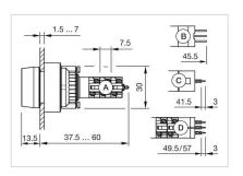
A = Solder terminal B = Plug-in terminal 2.8 x 0.5 mm
