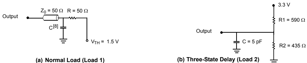
Figure 3. AC Test Load and Waveforms
