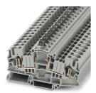
Component terminal block, If several diode terminal blocks need adding to the DIN rail, a spacer plate must be placed between them., with integrated P1000Y diode, nom. voltage: 1000 V, nominal current: 5 A, connection method: Spring-cage connection, Rated cross section:  $6~\text{mm}^2$ , cross section:  $0.2~\text{mm}^2$  -  $10~\text{mm}^2$ , color: gray
