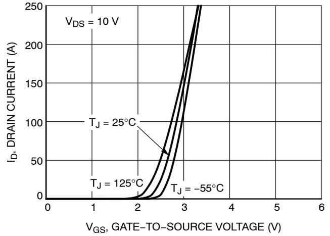
Figure 2. Transfer Characteristics
