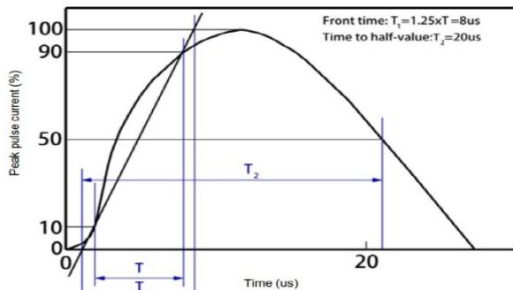
Fig 2 Contact Discharge Current Waveform per IEC 61000-4-2)
