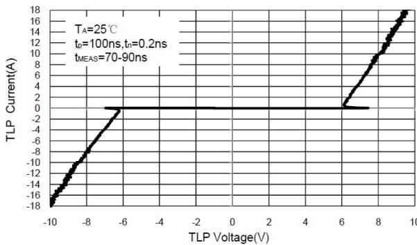
Fig 6 Clamping Voltage vs Peak Pulse Current
