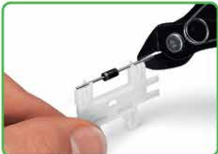
Cutting component to the proper length.
