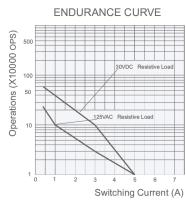
**Test conditions:** AgNi, Resistive load,  $85^{\circ}$ C, 1s on 9s off.
