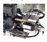
The combination of the Stripping Module with the AMP-O-LECTRIC Model G Terminator provides an economical and proficient method of stripping wire and crimping terminals on the same machine. Wires are stripped moments before crimping, meaning there is virtually no chance of damaging wire conductors during handling or storage. Once the wire is fed into the start sensor the Stripping Module does the rest, improving placement accuracy. Order Catalog 1309085 for more information.
