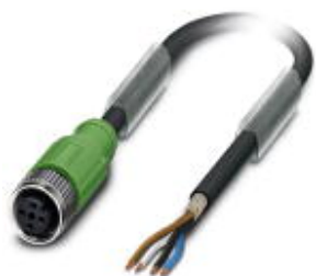
Sensor/actuator cable, 4-position, PUR halogen-free, black-gray RAL 7021, shielded, cable length: 5 m
