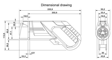
Make sure that the vehicle charging connector is placed in an appropriate charging connector holder, which ensures a minimum protection rating of IP24 in accordance with IEC 61851-1, for the entire time between charging. To create this charging connector holder, use the dimensions of the vehicle charging connector. Detailed dimensions can also be found in the Download area.
