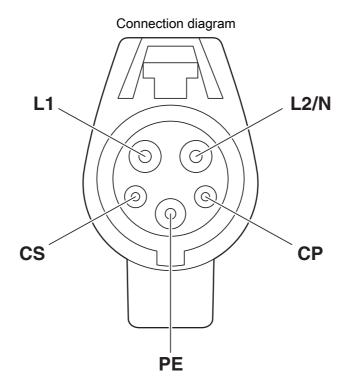
Pin assignment of the Vehicle Connector
