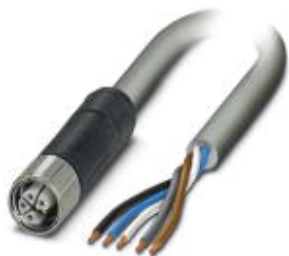
Power cable, 5-position, PVC, gray RAL 7001, Socket straight M12, L-coded, on free cable end, cable length: 10 m, for direct current up to 16 A/63 V
