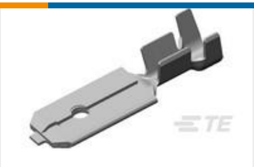
TE Part #626378-1 250 FASTON TAB 18-14 AWG BR
