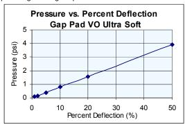
The resultant thickness of the Gap Pad will determine the thermal resistance. Subtracting the initial gap pad thickness by the deflection value, obtained above, will give the resultant thickness. Refer to the graph below to obtain the thermal resistance of the material.
