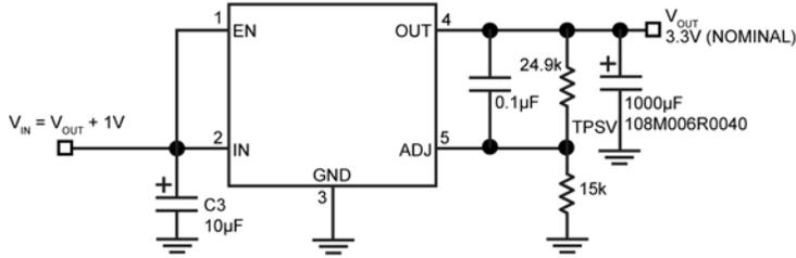
Figure 2. LT1764 Load Transient Response Test Circuit
