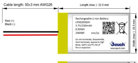
Thickness (max.): 5.0 mm (deliver status) 5.4 mm (after cycling)
