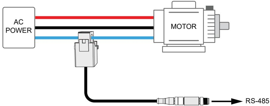
Installing a single conductor on the current transformer
