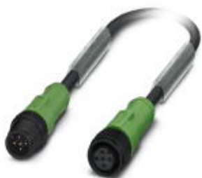
Sensor/actuator cable, 5-pos., PUR, halogen-free, black-gray RAL 7021, straight M12 plug, A-coded, to straight M12 socket, A-coded, cable length: 10 m, with plastic knurl
