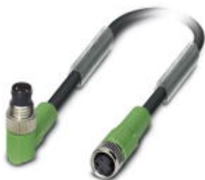
Sensor/actuator cable, 3-position, PVC, black RAL 9005, Plug angled M8, on Socket straight M8, cable length: 2 m
