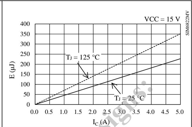
Figure 15-48. Low-side Switching Loss
