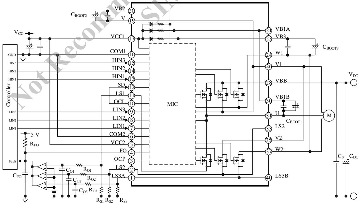
Figure 9-2. SIM6810M Typical Application Using Three Shunt Resistors
