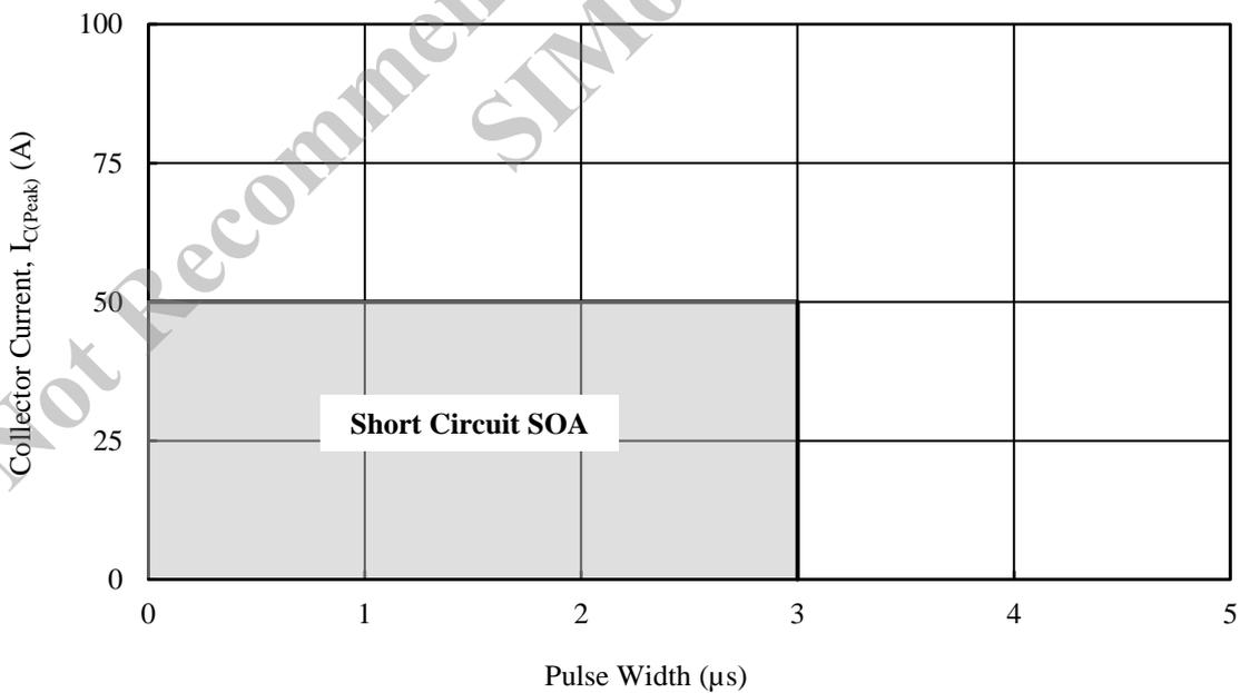
Figure 15-64. Short Circuit SOA: SIM6822MV, SIM6827MV
