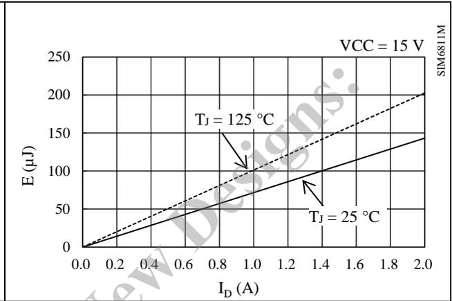
Figure 15-40. Low-side Switching Loss
