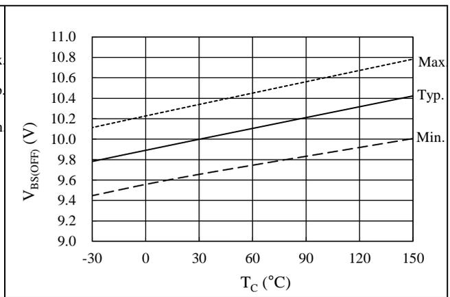
Figure 15-11. Logic Operation Stop Voltage,  $V_{BS(OFF)}$  vs.  $T_C$
