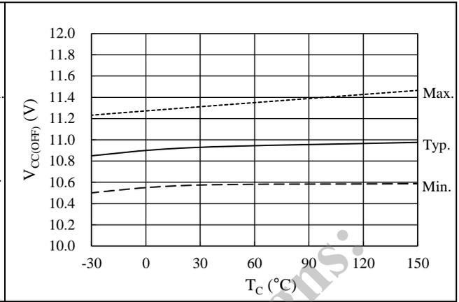
Figure 15-13. Logic Operation Stop Voltage,  $V_{CC(OFF)}$  vs.  $T_C$
