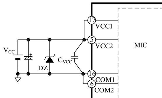
Figure 12-4. VCC<sub>x</sub> Pin Peripheral Circuit
