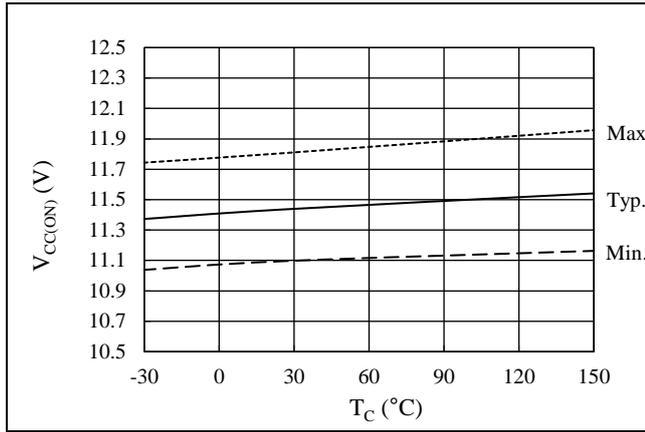
Figure 15-12. Logic Operation Start Voltage,  $V_{CC(ON)}$  vs.  $T_C$
