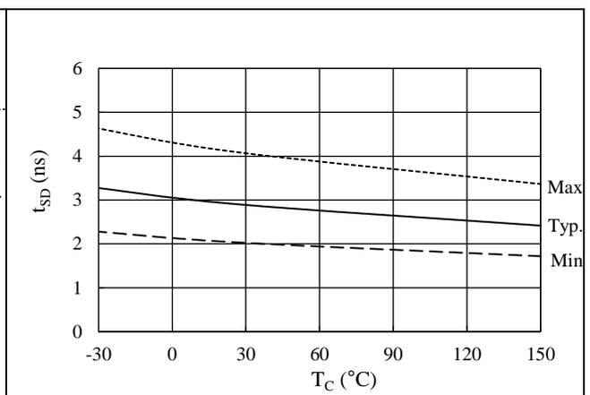
Figure 15-23. SD Pin Filtering Time vs.  $T_C$
