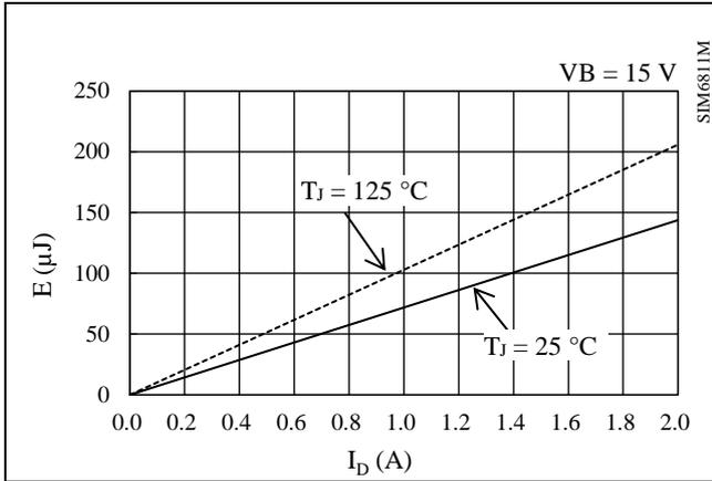
Figure 15-39. High-side Switching Loss
