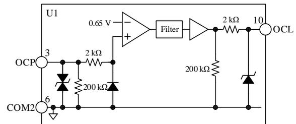
Figure 12-12. Internal Circuit of OCP and OCL Pins
