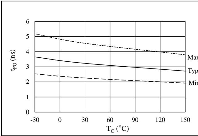
Figure 15-24. FO Pin Filtering Time vs. T<sub>c</sub>
