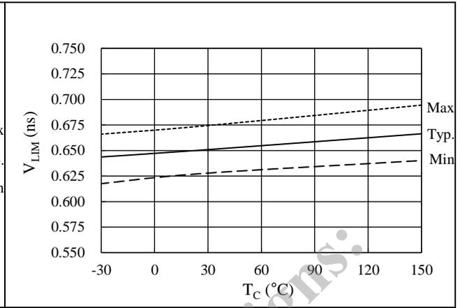
Figure 15-25. Current Limit Reference Voltage, V<sub>LIM</sub> vs. T<sub>c</sub>
