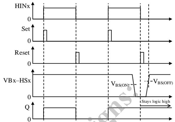
Figure 12-3. Waveforms at VB<sub>x</sub>-HS<sub>x</sub> Voltage Drop
