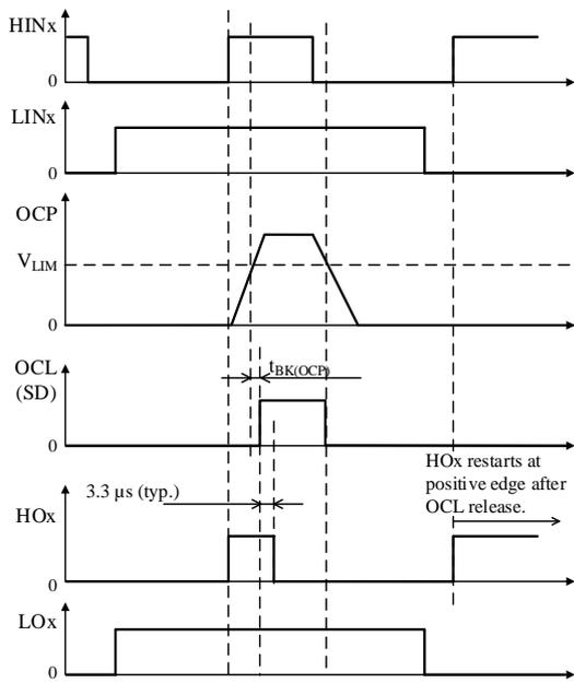
Figure 12-13. OCL Operational Waveforms (OCL = SD)
